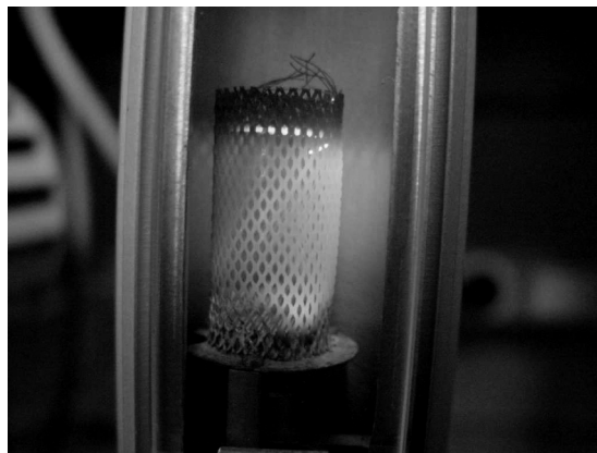
Fig. 7. A catalytic metallic net installed in the combustion chamber of hair-curlers.
