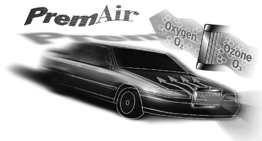
Fig. 2. Schematic drawing of the PremAir TM clean air systems.
